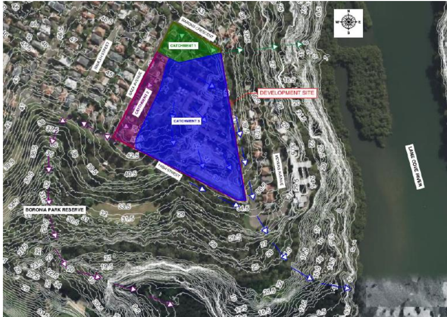
Figure 2 Existing stormwater sub- catchments
